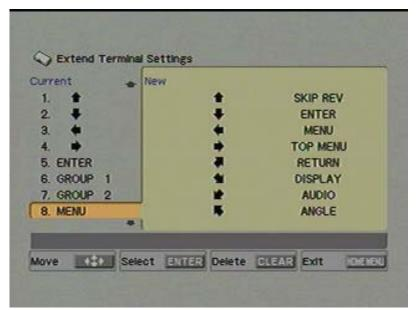
In order to DISABLE the switch function, please select the switch and Press "CLEAR" button. And then the switch will be displayed as "nothing" as shown below.
