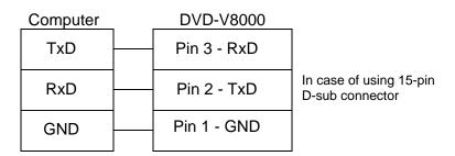
Some computers require the CTS port to be set to HIGH during communication. It is best to connect the CTS and DSR port on the computer to the DTR port on the player. During normal operation the player's DTR is set to HIGH thus the unit is able to receive a command at any time.
