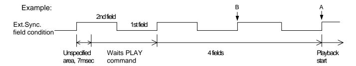
The video output under external synchronization delays for one field to the black burst signal input to EXT SYNC IN terminal. In the above figure, the field of black burst at the playback start timing is second field, but the field of the video output from DVD-V8000 is first field.
