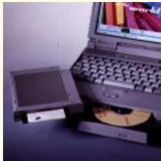
The Toshiba SelectBay: swapping between CD-ROM and floppy disk drives takes just seconds.
