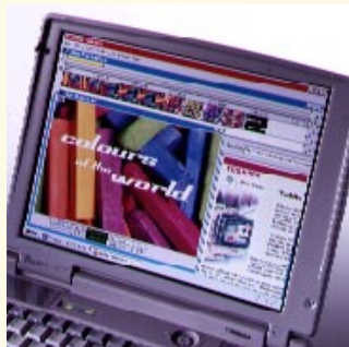
The 12.1-inch colour TFT screen has a resolution of 1024 x 768.
